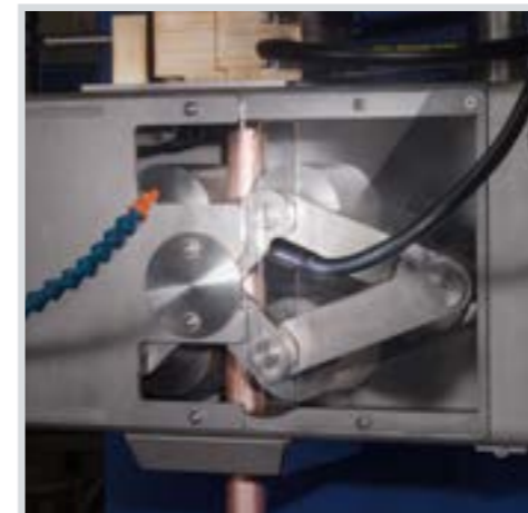
The Quattro Drive System with four feeding rolls. On left side in the foreground the additional secondary cooling system, on the right side the movable LED spotlight for easier feeding control.
