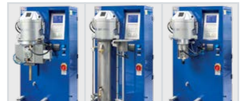
VCC 400 in continuous casting mode The same machine as granulating unit... ..and here equipped with the sintering kit
