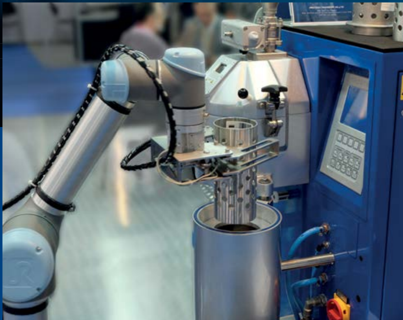
The VC 680 R special development has been specifically programmed and converted for use with robots.
