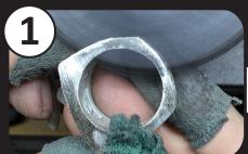
REMOVE SPRUES AND MATERIAL QUICKLY AND EFFICIENTLY!
